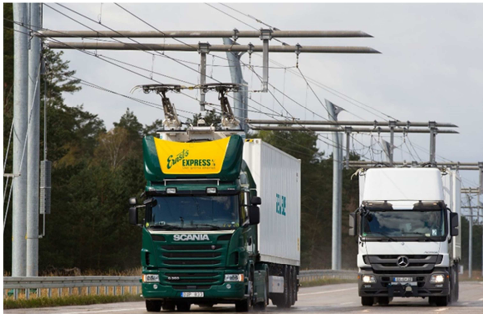
Figure 7: An example of conductive dynamic charging with two overhead pantographs (Source: Scania)
