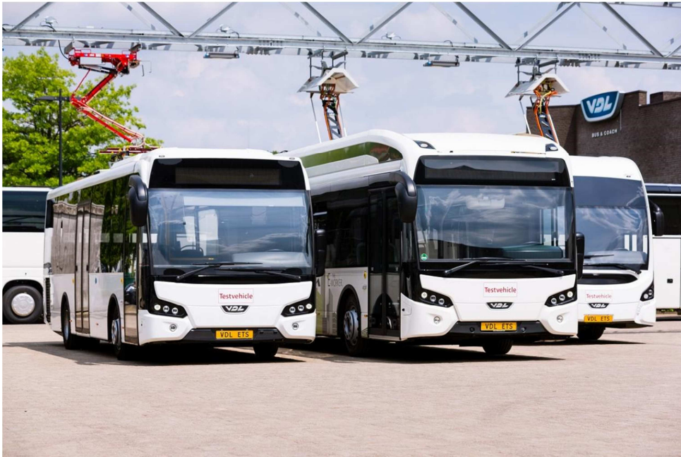
Figure 12: Inverted pantograph and rooftop pantograph ( http://www.vdlindustriesga.com/news/vdl-presents-unique-charging-plaza-in-valkenswaard )
