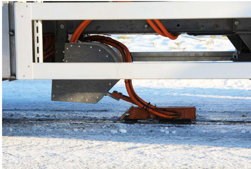
Figure 6: An example of conductive dynamic charging with a movable arm or a “ski” (Source: Dezeen)
