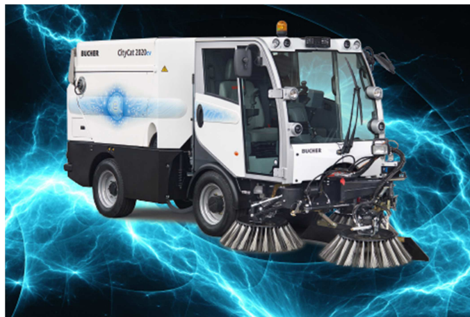
Figure 3: Bucher CityCat 2020ev battery electric street sweeper (picture: Bucher)
