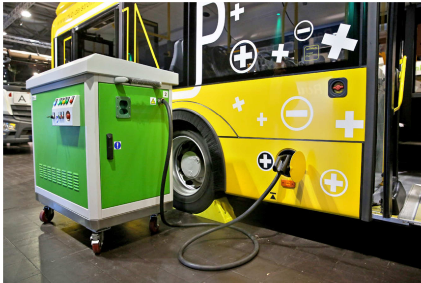
Figure 11: Charging Electric Bus with Depot Charger ( https://newmobility.news/2017/07/26/polish-electric-buses-brussels/ )
