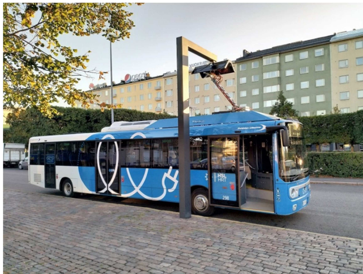
Figure 4: Electric bus charging at Hakaniemi charging point
