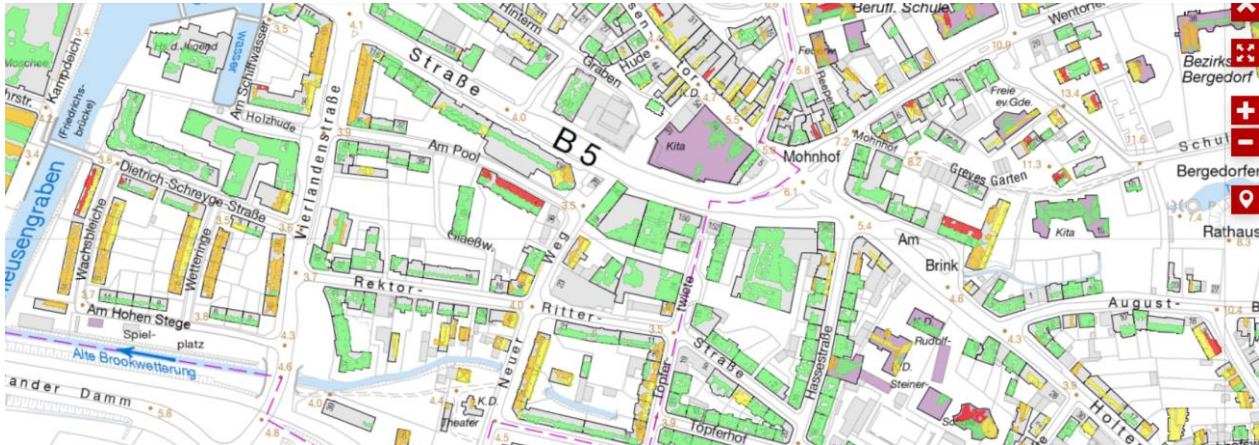
Figure 5-4: Screenshot of the “Solar-Atlas Hamburg”, Source: https://www.geoportal-hamburg.de/Solaratlas/index.html# In this potential analysis, 154 roofs with approx. 9,440 kWp were identified as suitable for PV power production according to the “Solar-Atlas” (see Appendix, Table 10-1). A range of roofs were eliminated based on further suitability criteria, e.g. less than 20 kWp possible power.
