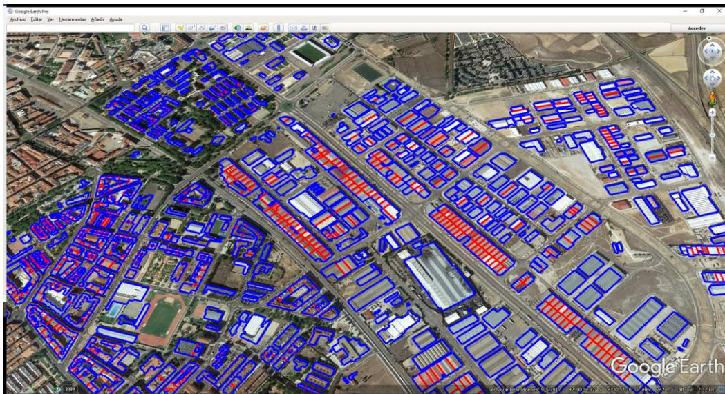
Figure 11 Building façades (in Blue) and adjoining walls (in Red) in Palencia study area
