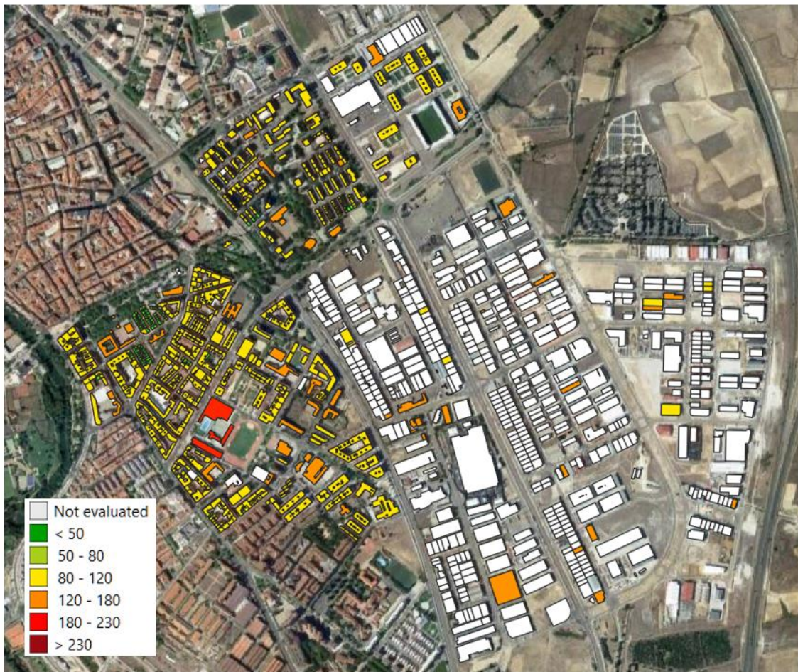
Figure 56 Total electricity consumption (kWh/m 2 ) of the district selected in Palencia
