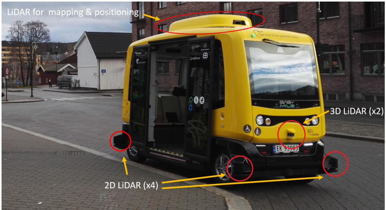
Figure 4: Easymile EZ10 Gen2 automated shuttle LiDAR radars [Ismailogullari 2018].
