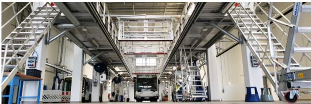
Figure 4: Second level roof workshop space within the e-bus workshop at VHH [source: VHH]
