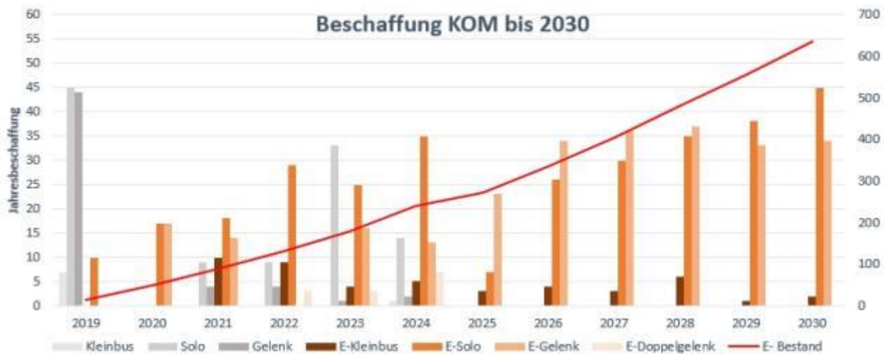
Figure 1: Forecasted scale-up of emission free vehicles at VHH (grey for diesel, orange for electrics) [source: VHH] The aim within the project was to both guarantee a high usability of the e-busses in operations through the largest possible range as well as preparing for a complete fleet roll-out. Interoperability of all systems also across other public transport providers especially within Hamburg as well as independence from the manufacturers to guarantee best results in future tenders was essential to the VHH focus.
