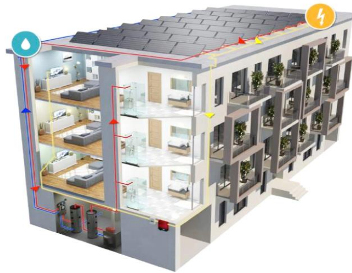
Figure 7: Implementation scheme in residential building for hot water preparation
