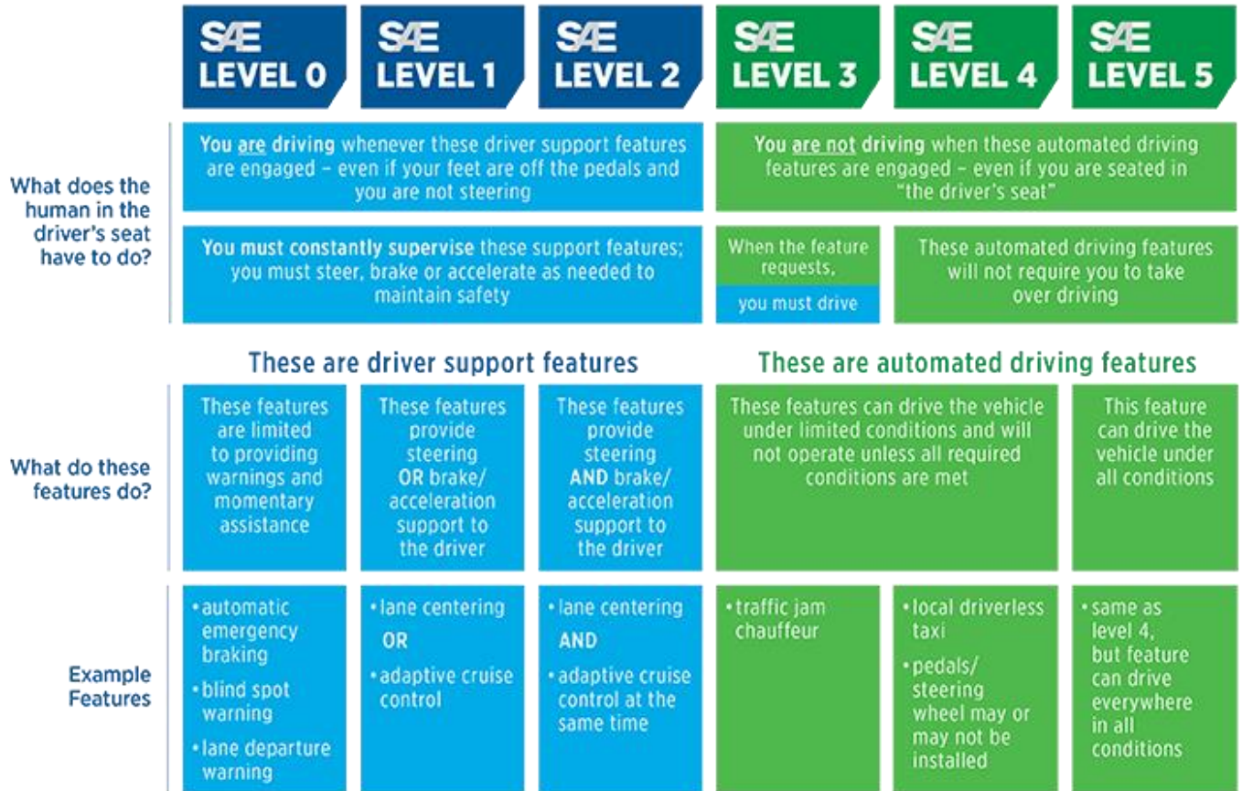
Figure 32: Levels of autonomous driving (Source: SAE website)
