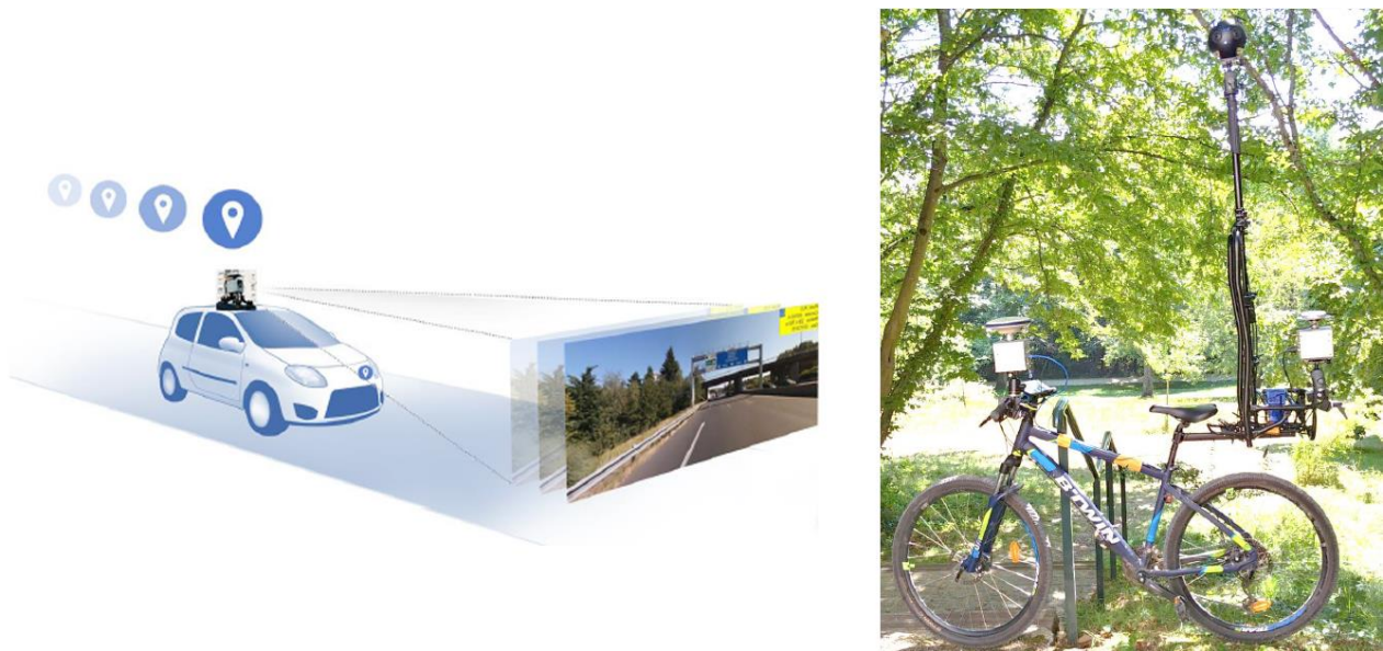
Figure 15: Installation on car (left) and bicycle (right) to collect data
