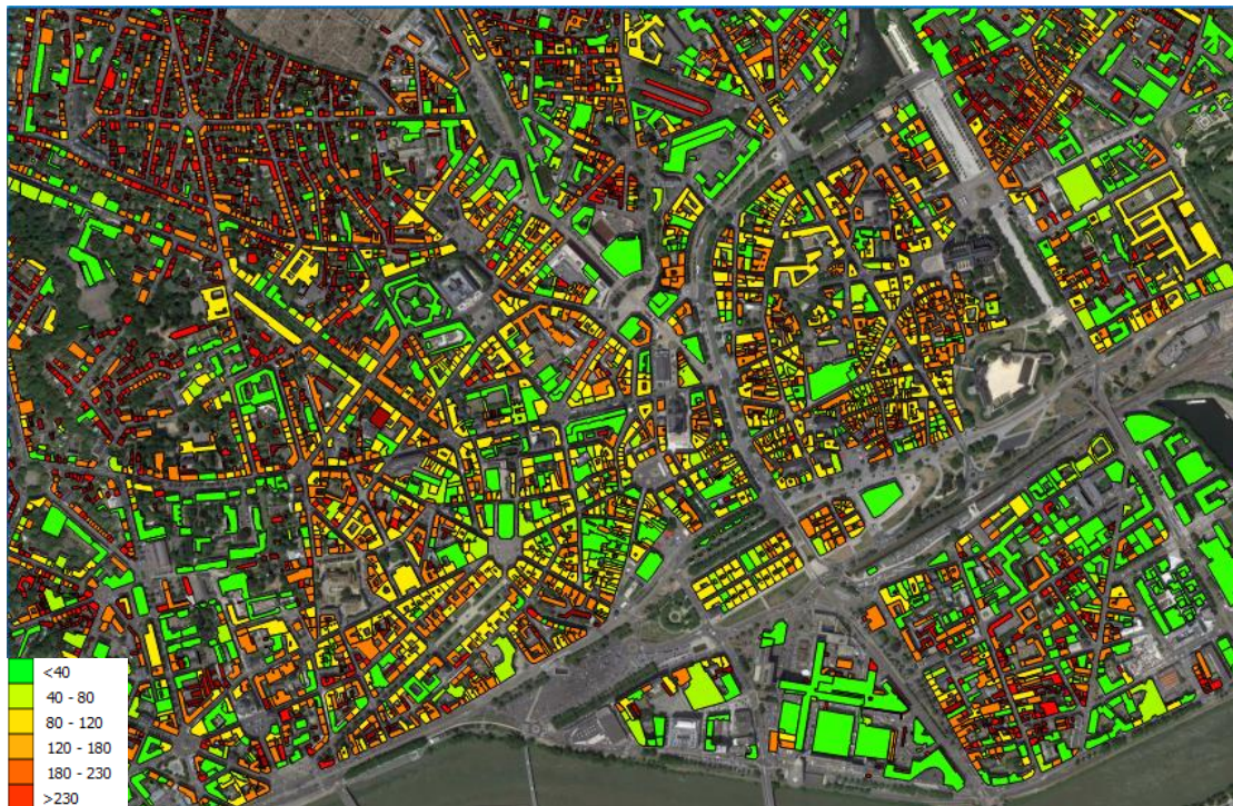
Figure 51: Heat demand (kWh/m 2 ) of a larger area of Nantes (the analysis has been carried out for the entire city of Nantes)
